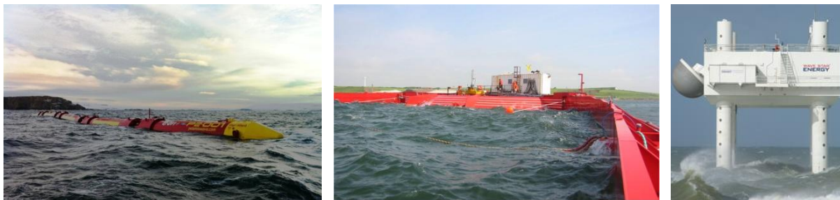
(a) (b) (c) Figure 23. (a) Prototype of Pelamis P2 in Orkney Islands (Pelamis, 2011), (b) Prototype of Wave Dragon in Nissum Bredning, Denmark (WaveDragon), and (c) Prototype of Wavestar at Hanstholm, Denmark (WaveStar).
