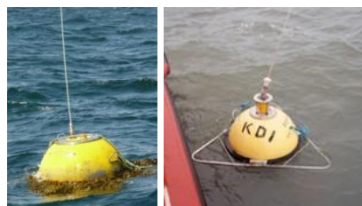
Figure 7. Waverider buoys installed at Galway Bay, Ireland (left) and at the Danish Coasts (Kys) (right).
